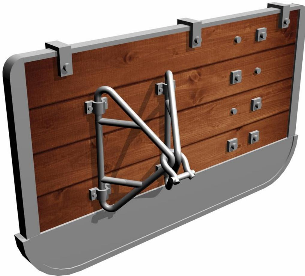
Flat wooden door. This is one of the earliest known designs of otter boards. Nowadays, in the UK, it is used mainly by smaller trawlers towing in shallow water. They are easily constructed and easy to maintain. In some fisheries, plywood is used instead of the wooden planks.
