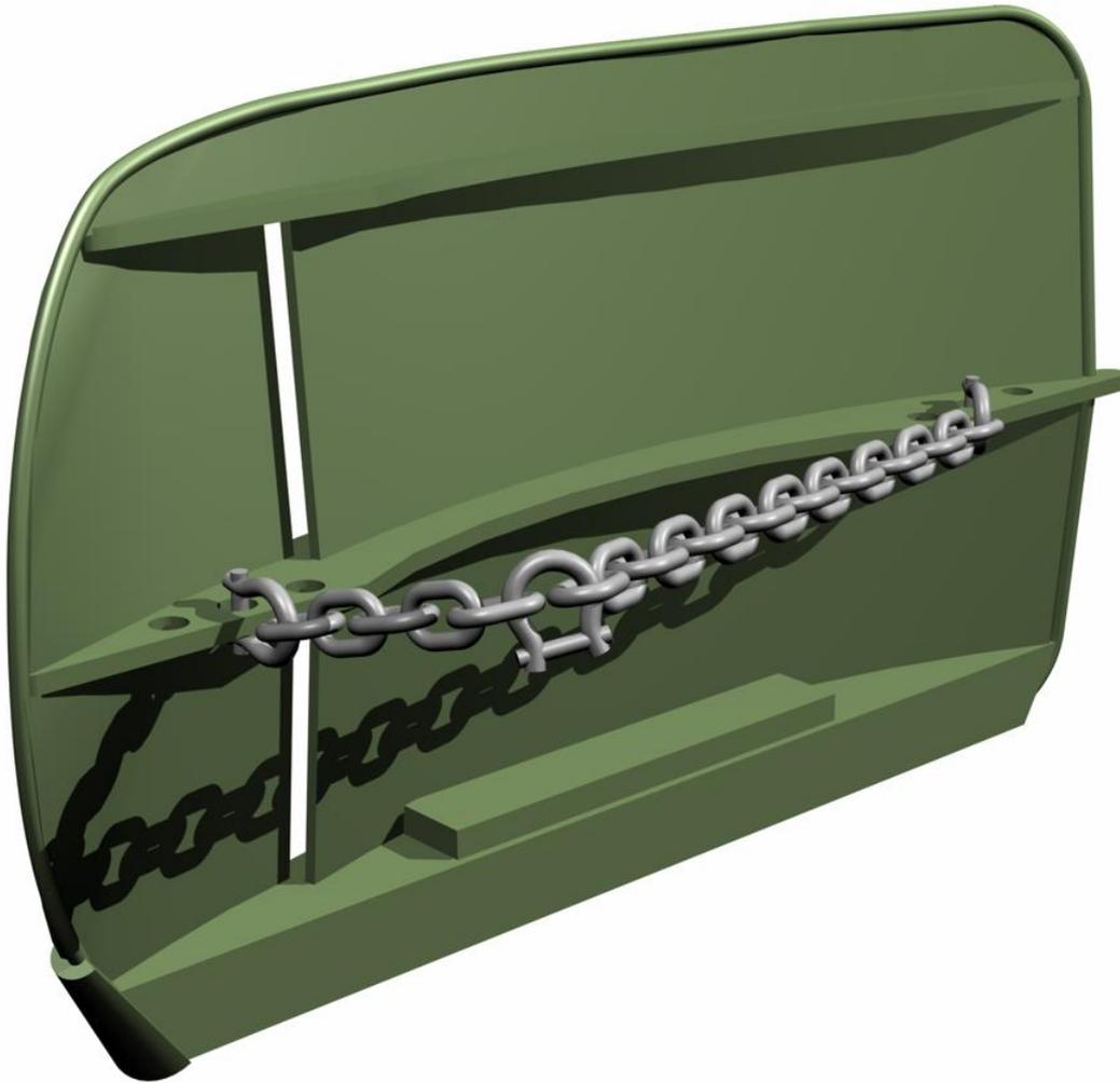
The idea of the curved plate is to improve water flow around the trawl door, thereby improving efficiency.
